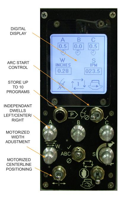
This advanced oscillation package is designed to increase production and improve the quality of the weld produced in automatic mechanized welding operations by minimizing weld defects such as poor penetration, incomplete fusion, overlap and undercut.
