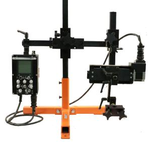
The remote control oscillator is ideal for use with a manipulator stand (KR-1000-WSB) and excels in pipe welding applications in combination with a weld positioner. \*support stand and bracketry sold seperatly
