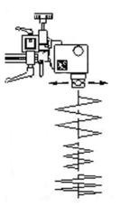
The weld oscillation head can produce a variety of welding patterns based on oscillation speed, dwell times and head or workpiece movement. The versatility and durability of the head makes the oscillator perfect for a variety of welding applications including, shipbuilding, tank welding, pipe welding, overhead welding and a list of other fabrication applications where weld oscillation is necessary.
